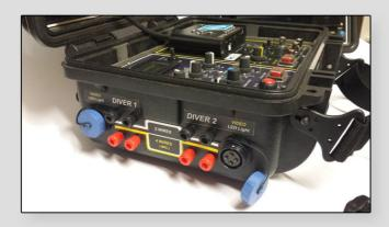
Outside there are, on one side the waterproof connectors for connection to the audio and video cables with the possibility of using the two-wire audio set for half duplex systems or the four-wire set for full duplex.
