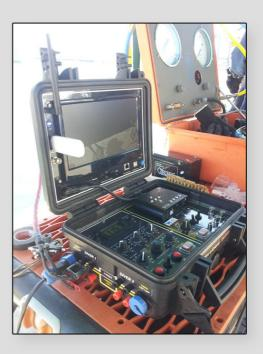
Two other unique features of the MINIEXPLORER Deluxe Plus are electronic protection to limit audio peaks that often cause the microphones and headphones in the helmets to break, and the restore communications system in full duplex mode in case of breakage of the same microphones.
